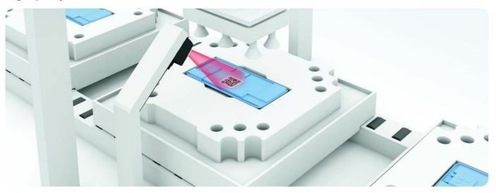
Smart Vision meet the increasing demands for maximum quality and great flexibility in modern manufacturing plants through integrated industrial image processing. With our BVS VisionSensor, optical quality control in automated production has never been easier. With its integrated and easy-to-configure image processing functions, the BVS VisionSensor meets the increasing demands for maximum quality and great flexibility in modern production systems.
