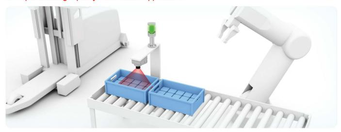
Digital industrial cameras with USB and Ethernet interfaces have an analog/digital converter, which makes a frame grabber superfluous and significantly simplifies handling. Thanks to the GenlCam, GigE Vision and USB3 Vision image processing standards, all cameras have standardized camera communication and unified naming conventions for camera functions and settings. This ensures easier operation.
